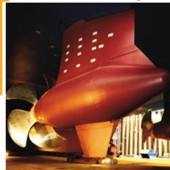
Radiance of the Seas , 2 x 19,5 MW Azipod® propulsion
