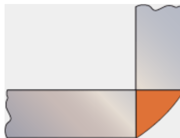
Corner joint fillet weld
